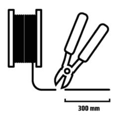
If the end cap has been absent or it is clearly damaged, cut 300 mm from the cable end and apply a new end cap.
