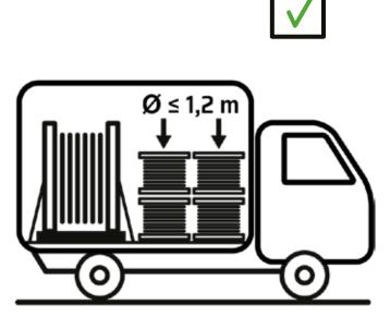
Secure the drums with a combination of wedges and transportation straps to tie down the drums during transportation. Drums with Ø≤1.2 m can be stacked.
