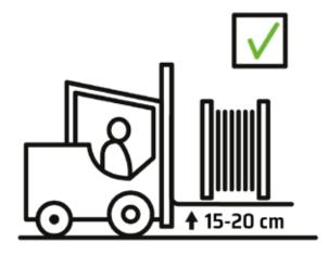
Lifting cable drums with a forklift is only allowed from the flange side.
