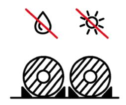
Cables with coloured outer sheaths shall not be stored in direct sunlight to prevent fading.
