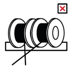
Cables should not be pulled crossing each other to avoid abrasion of the sheath at the crossing point.
