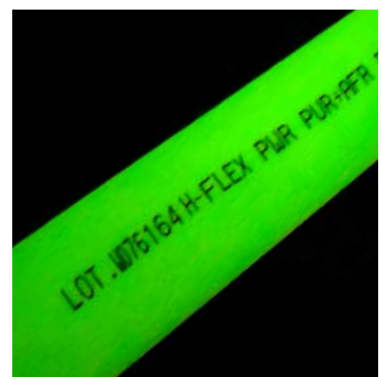
Luminous intensity test for luminosity after loading under light
