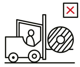
Never touch the cable or its protective cover with the forks.
