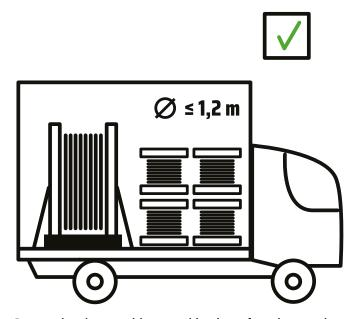
Secure the drums with a combination of wedges and transportation straps to tie down the drums during transportation. Drums with  $\emptyset \le 1.2$  m can be stacked.
