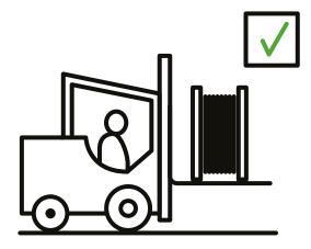
Lifting cable drums with a forklift is only allowed from the flange side.
