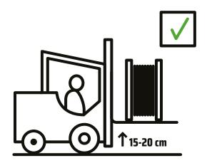
Raise the forks of the forklift sufficiently (15-20 cm) above the ground.
