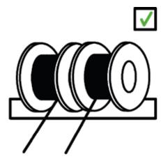
Only pull same size cables together. Use rollers when pulling big cables. The number of cables to be pulled at the same time is determined by the installation conditions at site: distance to be pulled, open space available for looping the cable at intermediary drawing stations, and the routing of cables (number of bends and number of corners).
