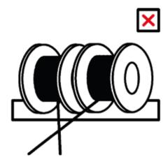
Cables should not be pulled crossing each other to avoid abrasion of the sheath at the crossing point.
