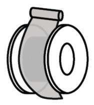
Plastic foil is wrapped over the cable layers and affixed with adhesive tape.
