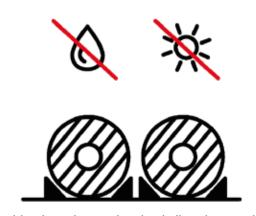
Cables with coloured outer sheaths shall not be stored in direct sunlight to prevent fading.
